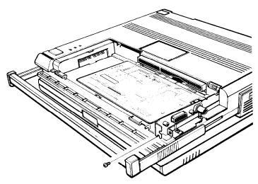
8. Set the cover on the computer and slide it back into position as shown below. Press firmly until the cover snaps into position.
